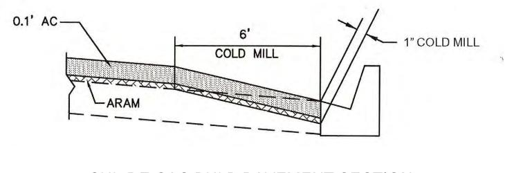
CUL-DE-SAC BULB PAVEMENT SECTION BEGIN AT BCR BEFORE BULB
