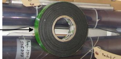
Sealing tape for baffle plate (green backing)
