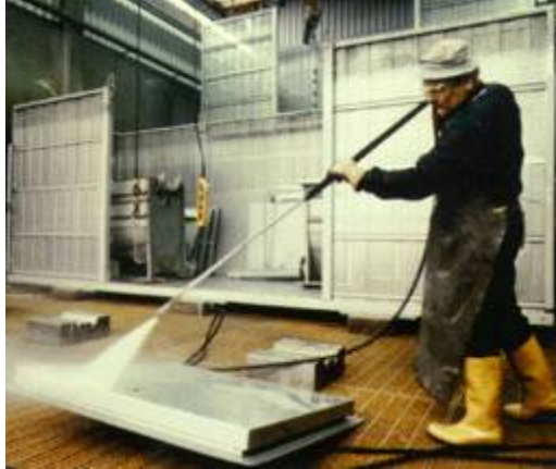
Image: Flushing and passivation after pickling process
