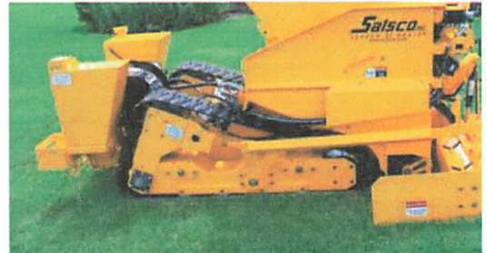
Tracks are fixed at 38" to accommodate screed style.
