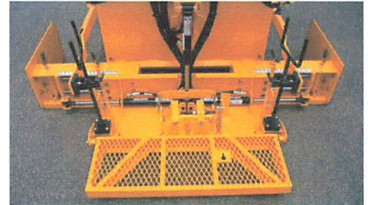
Hydraulic End-Gates move in & out, and have rulers on the top of the end gate to see where they are.
